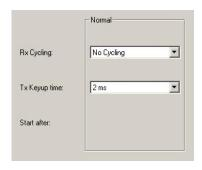
Receiver cycling can provide additional power saving by turning the receiver off and then on again for a brief period to check if there is a signal. Receiver cycling time is selectable with 0, 5, 10, or 20 mS options.
